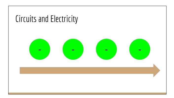
Electricity is just the flow of electrons. Electrons are tiny particles that every atom has. Electrons have negative charge, just like magnets where opposite charges attract and same charges repel. A circuit is a loop of conductive material (ie material that allows electrons to flow easily).
